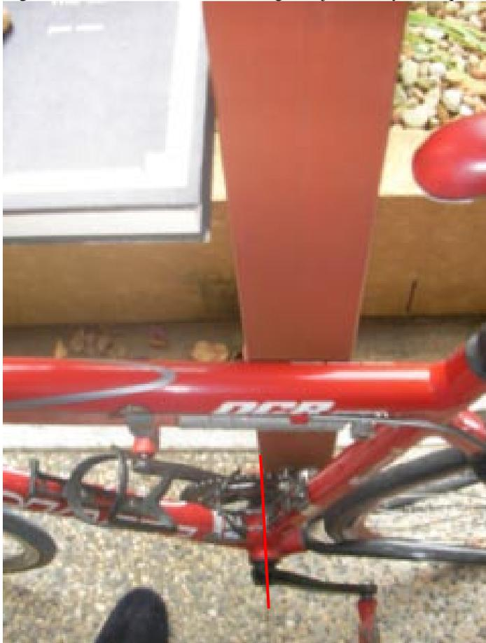
Ensure that the bike has not moved and is still aligned with the corner as per figure 7 then measure the distance from the tip of the saddle to the edge of the book or other straight object being used as shown in figure 9.
