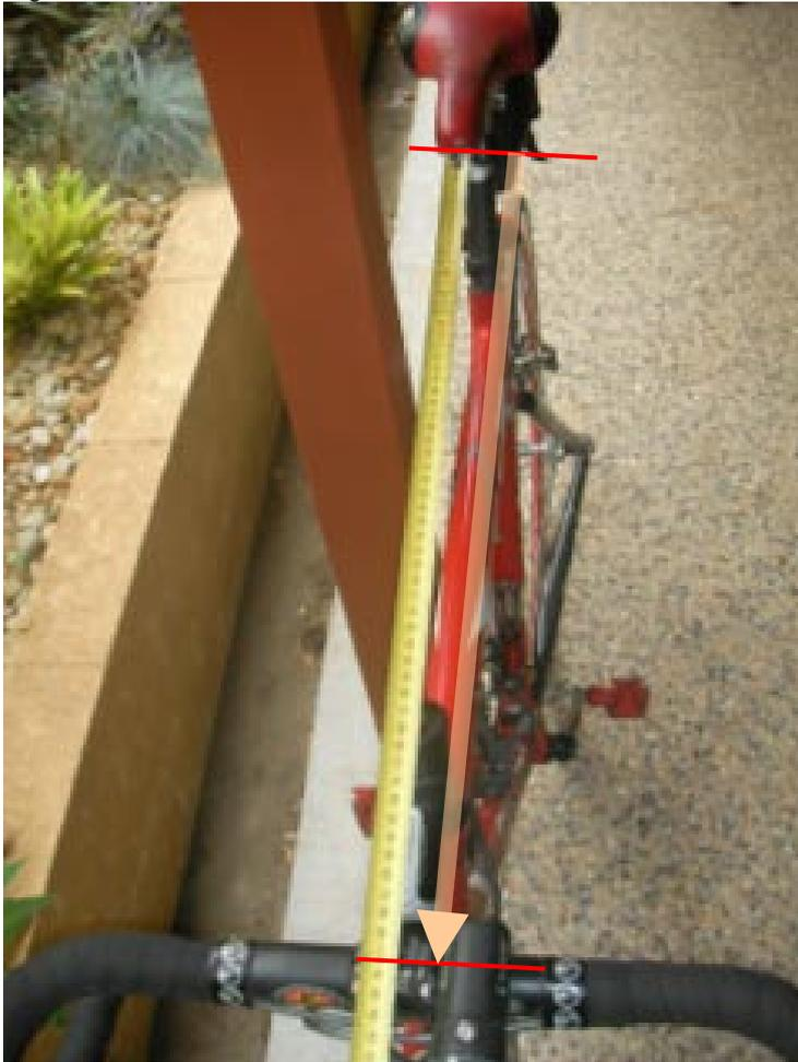
Figure 6: Take measurement at centre of stem clamp.
